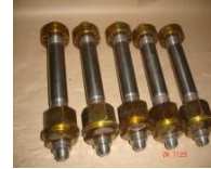
STUDS FOR GIRTH GEAR
