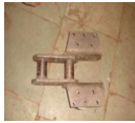
LINK OF ELEVATOR CHAIN 956
