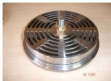
DISCHARGE VALVE OF O2 COMPRESSOR
